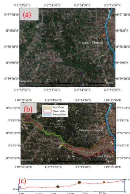
Figure 2: Lateral flow area in Juno Oge due to Donggala Earthquake, (a) before flow failure, (b) after flow failure with mud flow and water channel and (c) slope profile of the flow area (modified from Google Earth).
